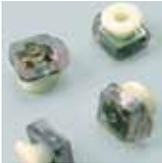
Standard nylon swivel glides are designed for maximum holding power, with an exclusive, double-tiered springsteel clip attachment with eight fingers and a clear vinyl bumper/boot for better stacking and finish protection. Tested to exceed 300 lbs of pulling pressure.
